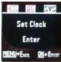
**SETTING THE CLOCK:** Scroll over to the **SYS** tab using the ► ◀ buttons and then press the ▼ button to enter the **Set Clock** option. Press **OK**. You will see the following screen. (Fig 11)
