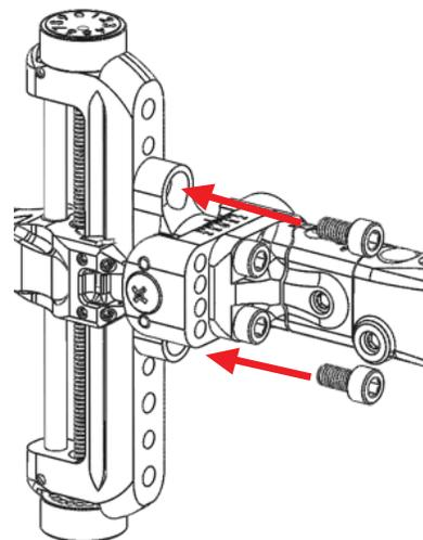
3. Attach the Mounting Bracket (D) to your bow using the two 10-24 x 1/2" Flat Head Socket Screws (E) and the 1/8" Hex Key Wrench (H). The Mounting Bracket can be installed with the knob up or down, depending on your setup.
