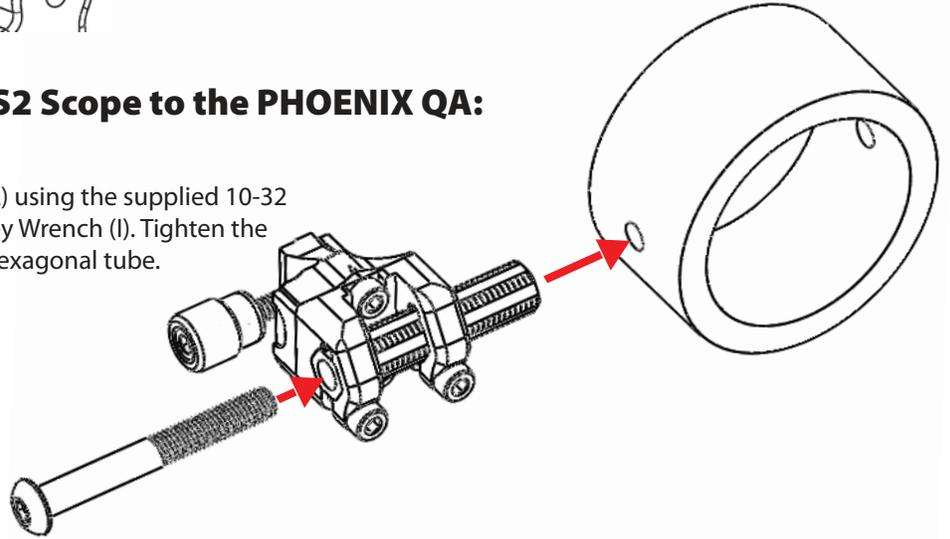
2. Use the PHOENIX QA Quick Connect Knob (N) to secure the Scope Leveling Mount (L) and Scope to your PHOENIX QA. Tighten the knob until the Scope Leveling Mount is secured in place.
