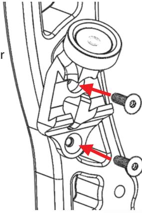
4. Attach your scope/aperture to the PHOENIX QA, (See directions following this section) and slide the PHOENIX QA Extension dovetail into the Mounting Bracket. Choose which detent in the extension best fits you, and tighten the Mounting Bracket knob to secure the PHOENIX QA in place.
