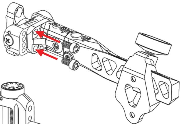
2. Attach the PHOENIX QA Elevation Frame (C) to the PHOENIX QA Windage Assembly (B) as show, using the remaining two 10-32 x 3/8" Socket Head Cap Screws (F), and the 5/32" Allen Wrench (I). A good starting point is to position the PHOENIX QA Windage Assembly near the center of the frame, though moving the PHOENIX QA Elevation Frame up or down may be necessary depending on your setup.
