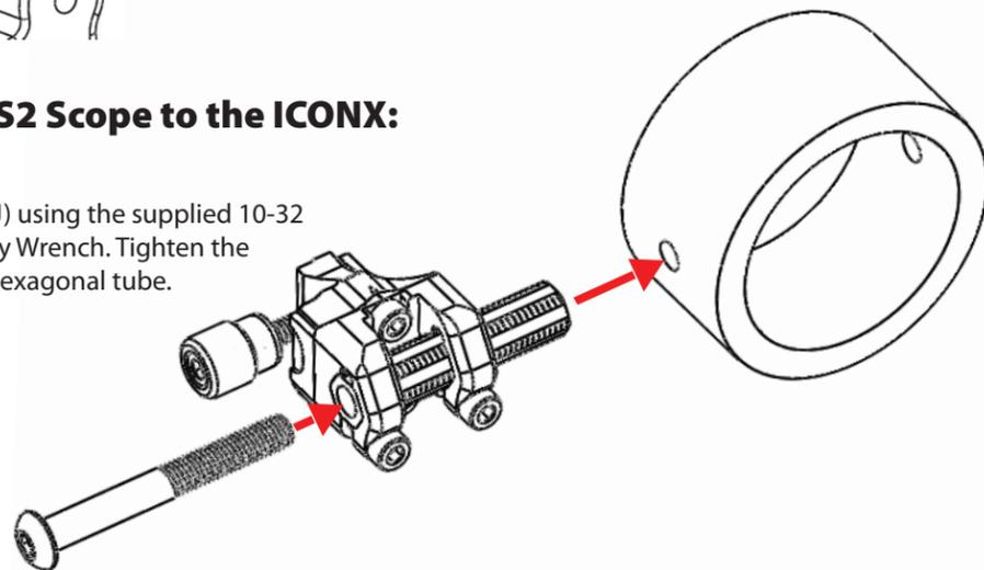
2. Use the ICONX Quick Connect Knob (L) to secure the Scope Leveling Mount (J) and Scope to your ICONX. Tighten the knob until the Scope Leveling Mount is secured in place.
