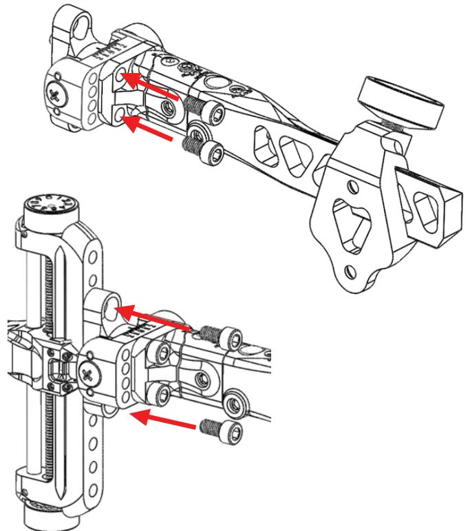
3. Attach the Mounting Bracket (D) to your bow using the two 10-24 x 1/2" Flat Head Socket Screws (E) and the 1/8" Hex Key Wrench. The Mounting Bracket can be installed with the knob up or down, depending on your setup.
