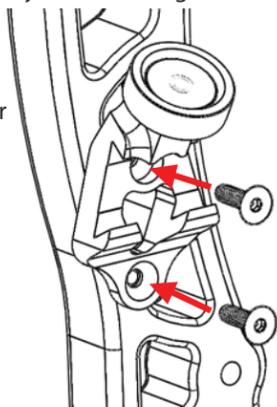
4. Attach your scope/aperture to the ICONX, (See directions following this section) and slide the ICONX Extension dovetail into the Mounting Bracket. Choose which detent in the extension best fits you, and tighten the Mounting Bracket knob to secure the ICONX in place.
