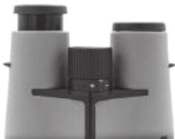
The eyecups may be personalized for your viewing comfort. Pull the eyecups all the way out for viewing without eyeglasses or collapse all the way in when wearing glasses. When wearing glasses, it is common for users to rest the rubber eyepiece directly against their eyeglasses.
