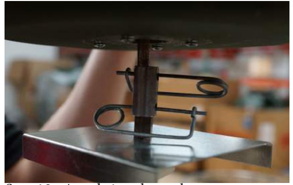
Step 10: Attach 1 end coupler to motor attach other end to auger. Insert safety pins.
