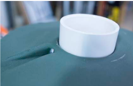
Step 5: Place PVC in hole and attach.
