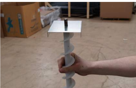
Step 7: Place spinner on top of auger.
