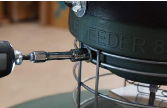
Step 11: Bolt powerhead down.
