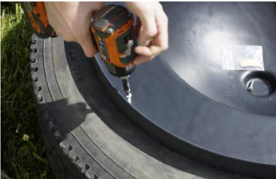
Step 3: Attach base to tire. (4) Tire screws
