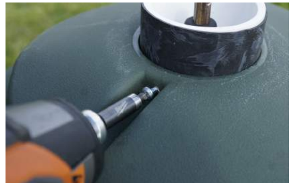
Step 6: Place PVC in hole and attach. (1) Set Screw
