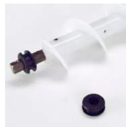
(1) Rubber Coupling on Auger
