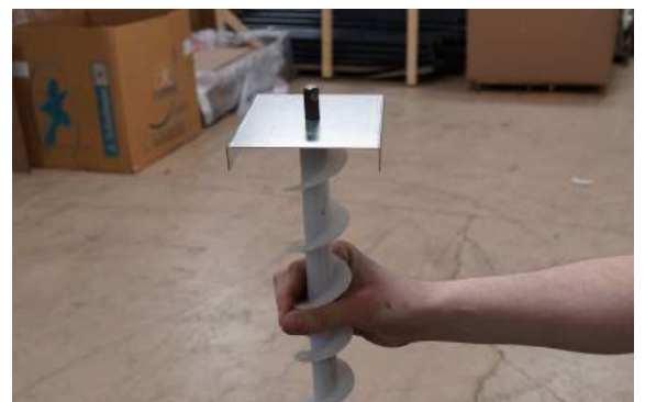
Step 8: Place spinner on top of auger.
