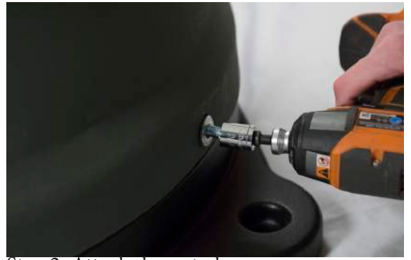
Step 2: Attach dome to base. (4) SM Washer (4) Bolt
