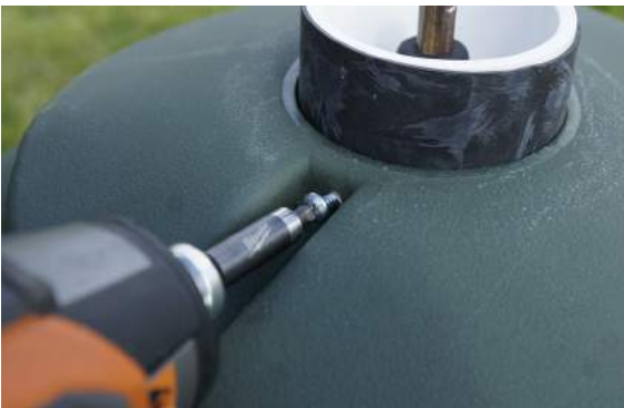
Step 5: Place PVC in hole and attach.
