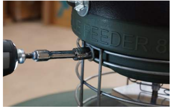
Step 10: Bolt powerhead down.
