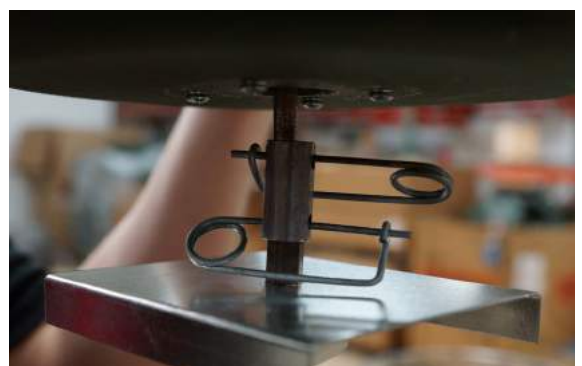
Step 8: Attach 1 end coupler to motor attach other end to auger. Insert safety pins.
