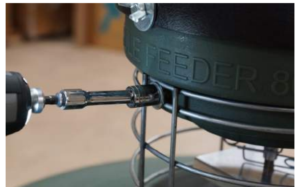
Step 14: Bolt powerhead down. (3) SM Washer (3) Bolt
