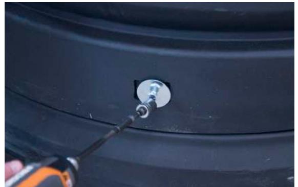
Step 4: Attach extension ring to base.
