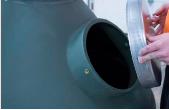
Step 9: Attach fill cap (2) Wing Nut
