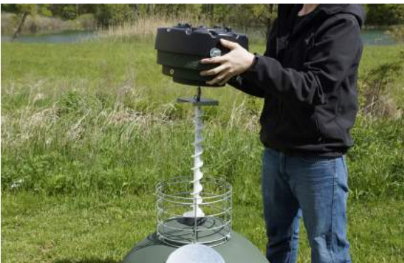
Step 13: Place powerhead on top of cage.
