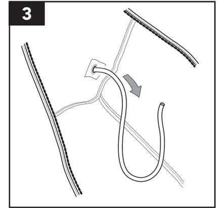
3 Pull the hose through the hole from the inside of the bag.
