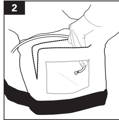
2 Feed the hose through the hole located on the inside of the pouch.
