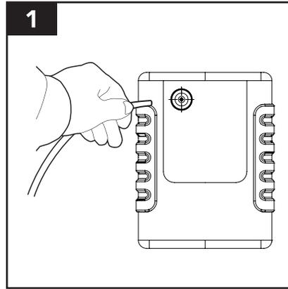
1 Attach the hose to the Ozone Machine. The hose will transport the ozone from the machine into the bag.
